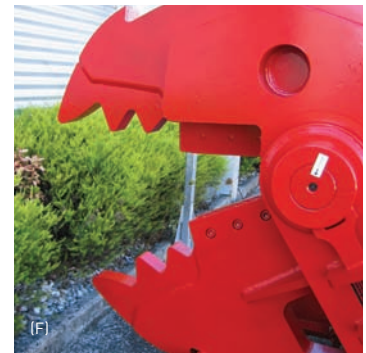
IMAGES: (D) Removing suspended floors: (E) & (F) Close view of Concrete Shear Jaw
